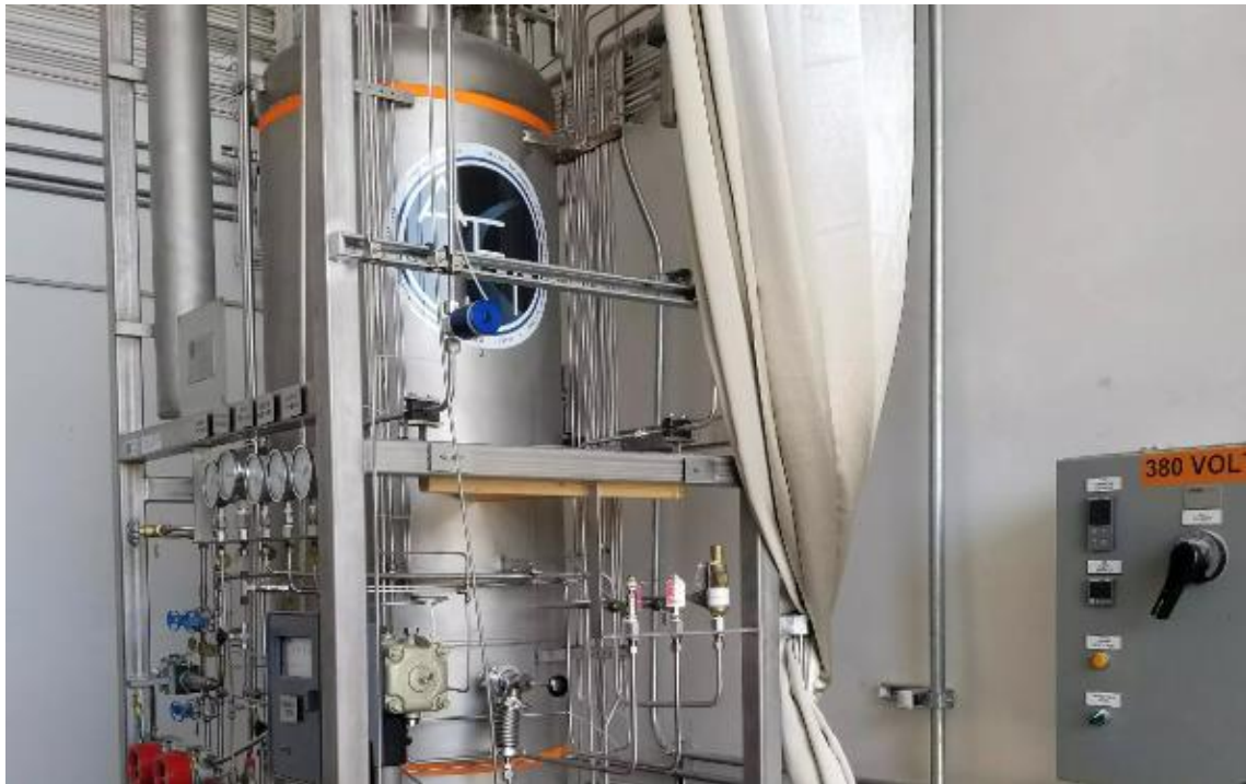
Figure 14.9: Hydrogen impurity temperature-swing adsorption column offered by Ability Engineering [50]
